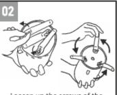
Loosen up the screws of the folding legs at the bottom of the stove body, extend them outwards in the right position, so as to maintain the stove body stable, and fasten them up again. It is advisable to use Pyrolino when the folding legs are extended, as it can damage sensitive surfaces.
