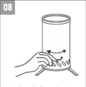
Adjust the flame density controller (-+) accordingly, depending on the type of fuel you use.
